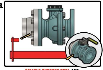
REMOVE SUPPORT TOOL AND INSTALL THE LAST TWO BOLTS
