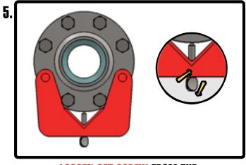
LOOSEN SET SCREW FROM THE BOTTOM OF THE FLANGE
