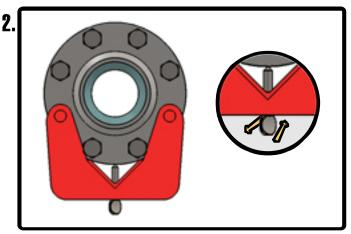
TIGHTEN SET SCREW INTO THE BOTTOM OF THE FLANGE LOCKING THE SUPPORT TOOL TO THE FIXED FLANGE.
