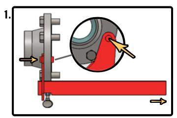
**INSERT SUPPORT TOOL INTO BACK SIDE OF FLANGE**
